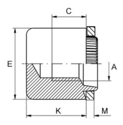
Female thread A = M3Height K = 9.0Min thread length C = 3.0Outer diameter E = 8.0Plate thickness = 4.7 to 4.9
